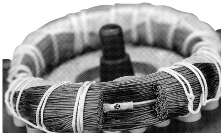
PTC sensor incorporated in windings
